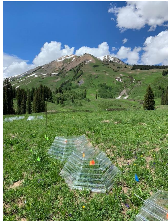
Open-top warming chambers (OTCs) deployed in a subalpine meadow near the Rocky Mountain Biological Laboratory
