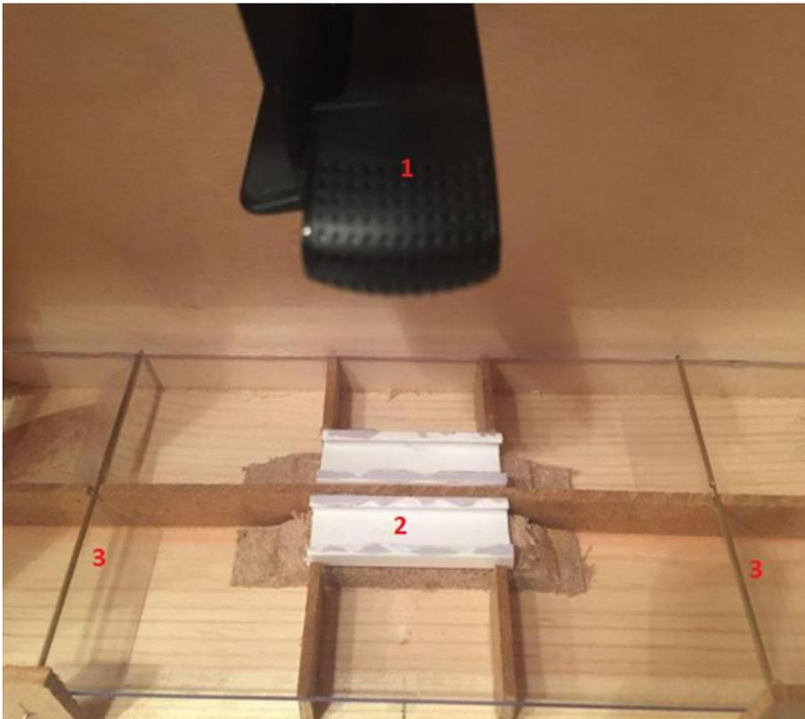
**FIGURE 2.** A close-up picture of the inside of the monitoring box, showing the main components. A camera (1) placed directly above a chokepoint (2), which was designed to slow down passing bumblebees. A pair of one-way doors (3) was installed in both tunnels to separate bumblebees entering and leaving the colony.
