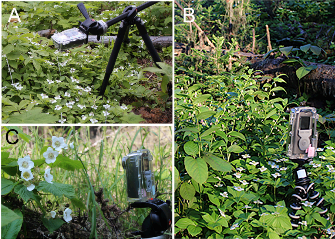
Appendix Figure I. Time-lapse camera set-ups: A. the Brinno 200 Pro HDR on a tripod filming a patch of Cornus canadensis (Cornaceae), B. the Brinno 200 Pro HDR on a GorillaPod (Joby, San Francisco, California) filming the bell shaped pink flowers of Streptopus lanceolatus (Convallariaceae), and c. the Brinno 200 Pro HDR on a tripod filming Rubus parviflorus (Rosaceae) Tripods were left in the field for the duration of the filming period and the cameras set out from 0900 to 2100 hours. This ensured that the same flowers were filmed each day.
