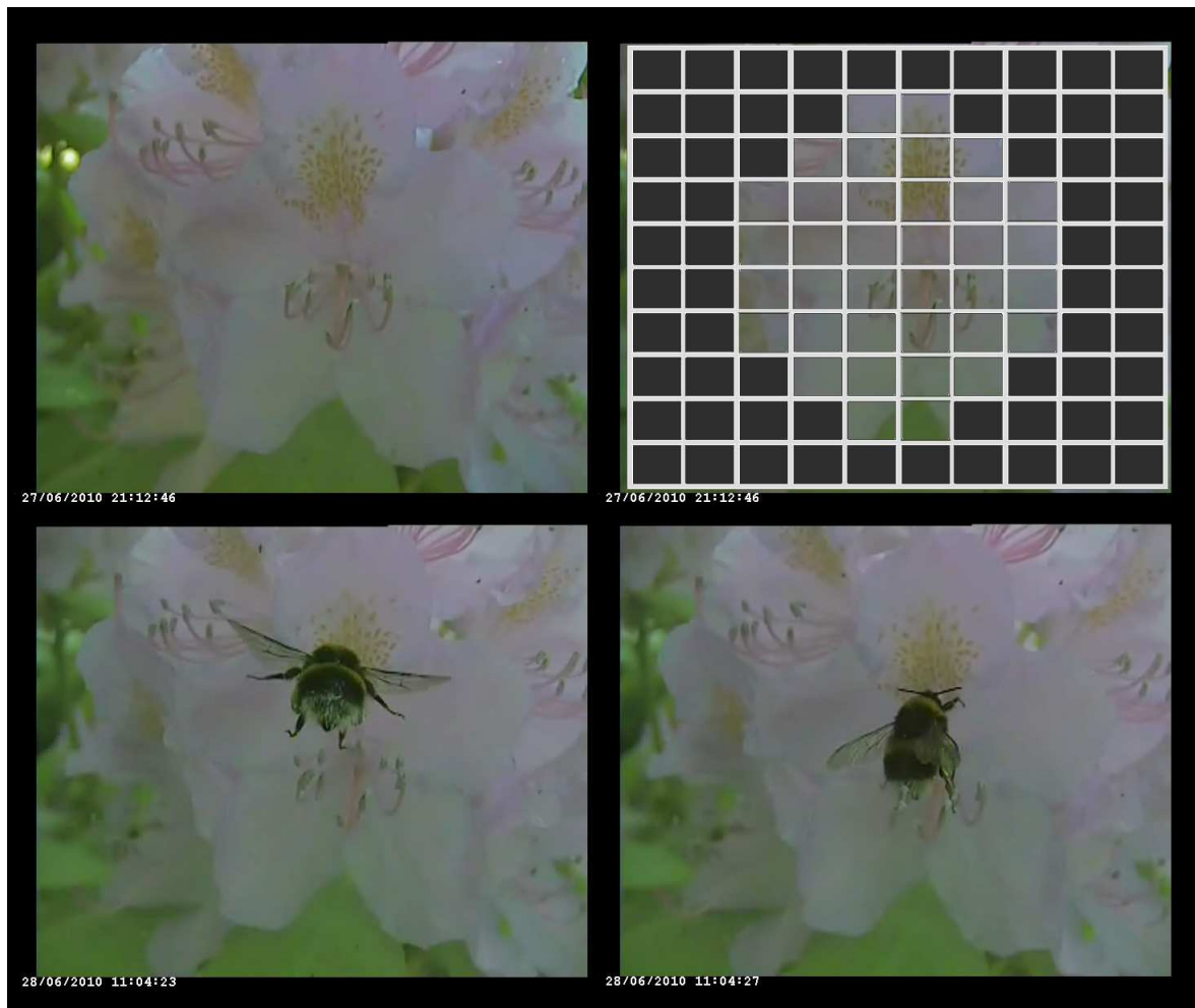
FIG. 2. Screenshots from recordings made of the rhododendron illustrating the video motion detection sensor. The upper left picture shows the camera view of the capitulum. The upper right picture shows the area that was masked (i.e. the dark grey square boxes). Only the unmasked area is sensitive to movements and triggers the recordings. In the lower left picture the approaching bumblebee that triggers the recording. In this case (picture lower right) it was classified to B. terrestris / B. lucorum group.
